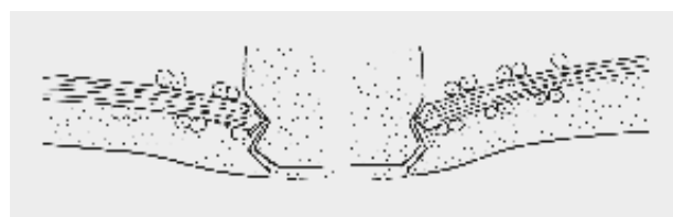
4 a–b Corvey, Church of SS Stephen and Vitus, external crypt from Phase I, reconstruction of the vaulted ceiling in the upper level, section (a) and detail showing joint in the plasterwork (b; drawing by Gerald Großheim)
