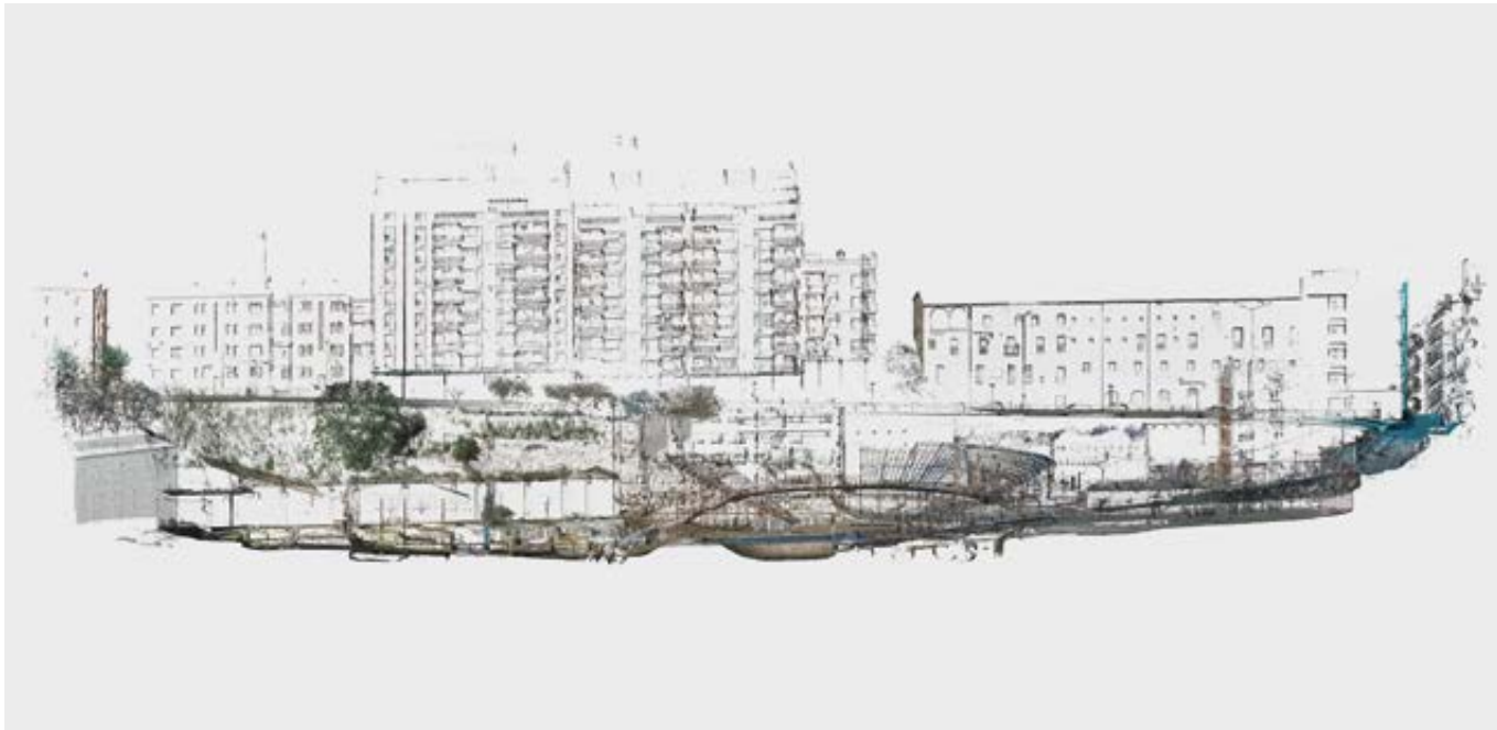
17 Laser scanner point cloud of the Roman Theatre created by technicians from the Architectural Heritage Service of the Generalitat of Catalonia.
